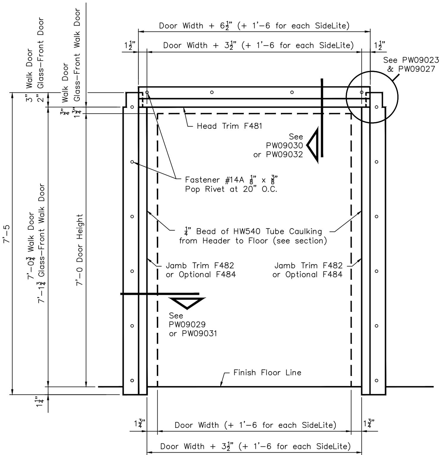
**Note:** All trim is to be installed BEFORE blanket insulation is applied to walls.
